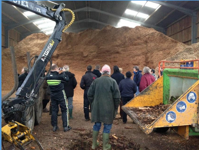
Dartmoor Woodfuel Co-operative's wood chip store. Due to its relatively low energy content when compared to gas or oil, wood chip fired systems need substantial space to store fuel. This can be a benefit to the project, however, if you have space available and can supply other installations. Photo Credit: Regen SW
